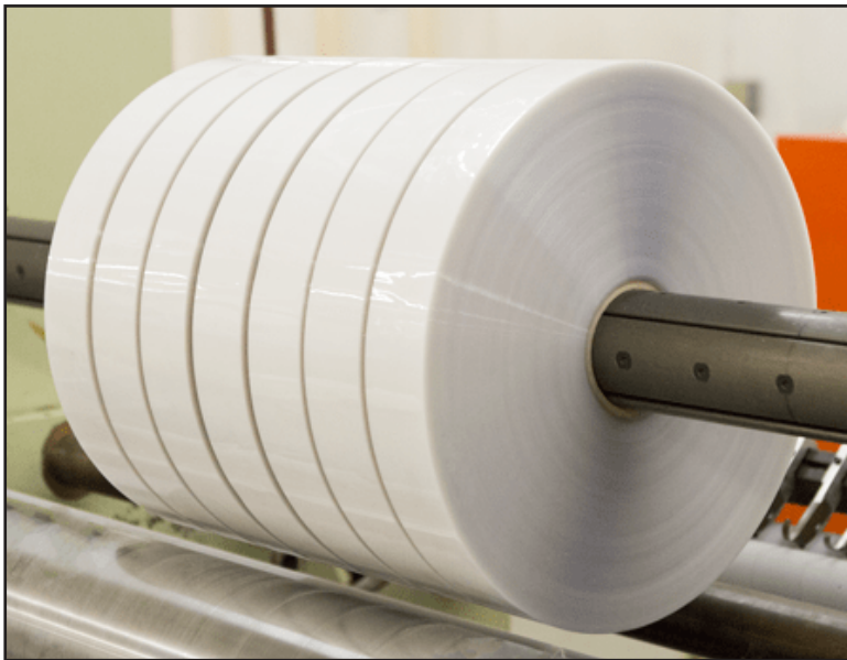
Slit cut rolls cut from large master roll of tape
