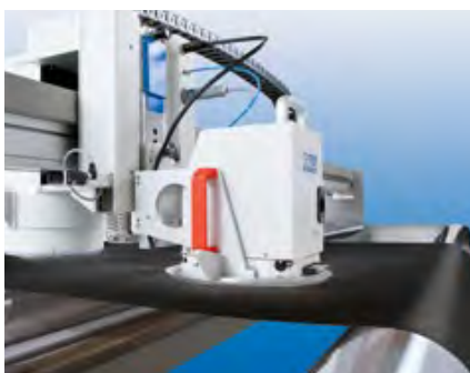
In-line testing of air permeability
