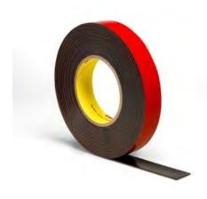
3M™ Acrylic Plus Tape Series EX4000 is a family of black, double-coated acrylic foam tapes designed for the attachment of automotive exterior trim parts such as body side moldings and claddings. 3M EX4000 tapes offer an advanced adhesive system that adheres well to traditional, low surface energy, and scratch- and mar-resistant automotive paint systems.
