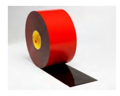
3M™ Acrylic Plus Tape Series EX4500 is a series of deep black, double-coated acrylic foam tapes designed for the attachment of automotive exterior trim parts – without the use of adhesion promoter. 3M series EX4500 tapes offer an advanced adhesive system – on both sides of the product – that adheres well to traditional, medium surface energy, and scratch- and mar-resistant automotive paint and polymer systems. The initial product offering will be in the 45 mil (1.1 mm) caliper.
