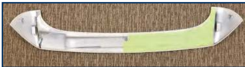
Molded spoiler - left half with hand-cut masking strips, right half with die-cut 3M™ 401+
